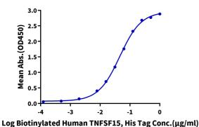
Immobilized Mouse DR3, His Tag at 1  $\mu$ g/ml (100  $\mu$ l/well) on the plate. Dose response curve for Biotinylated Human TNFSF15, His Tag with the EC50 of 45.6 ng/ml determined by ELISA (QC Test).
